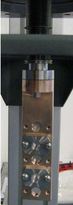
Figure 5. BL11-NCD: The support for the attenuators.
