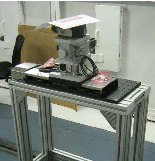
Figure 6. BL11-NCD: The lens support assembly housing the collimating beryllium lens for the micro-focus option.
