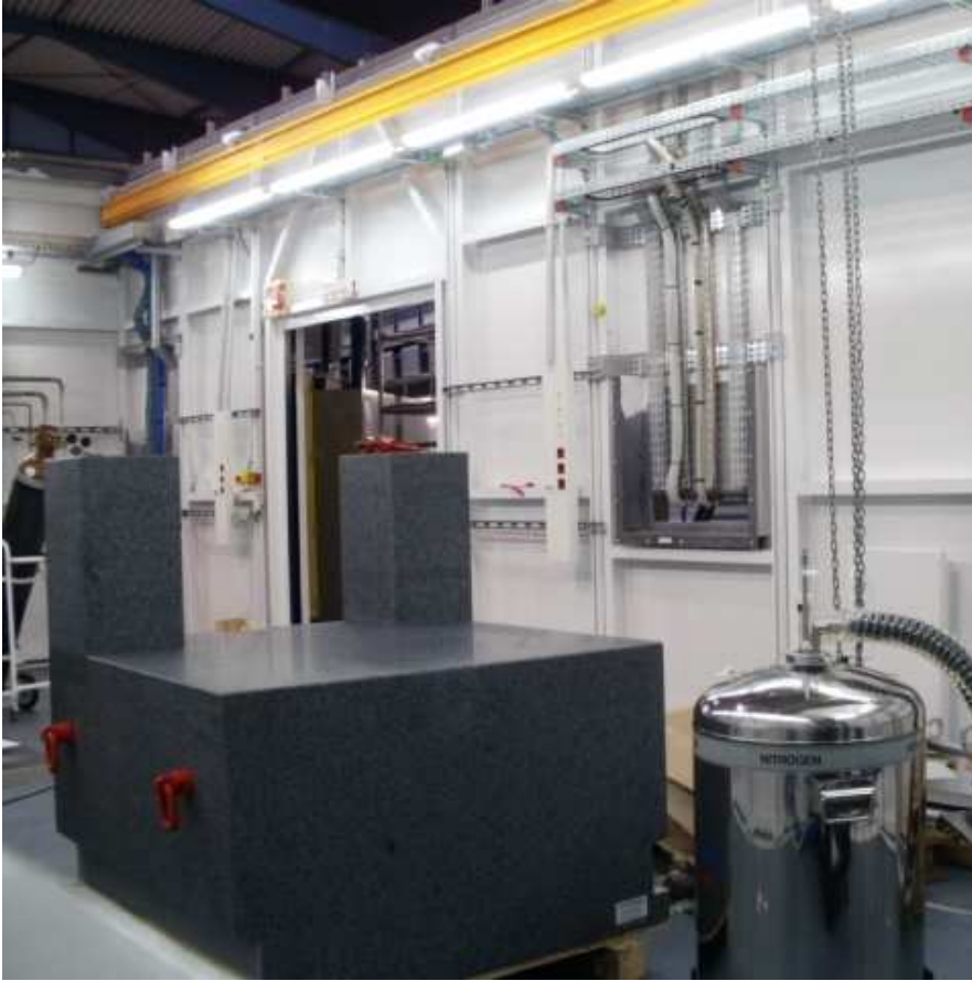
Figure 4. BL04-MSPD: High Pressure (HP) end station granite in the experimental hut.
